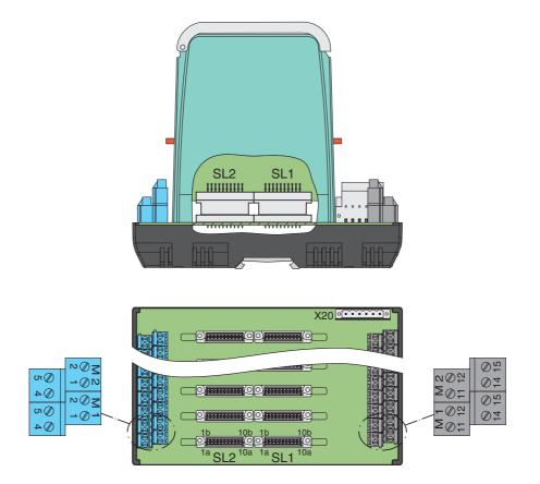
Insert the isolated barrier on the Termination Board. This closes the signal circuit between field side and control side. Connect field devices and controller to the terminals or connecting plugs of the Termination Board. For pin assignment between terminals, connecting plugs and connectors SL1/SL2, see drawing "Connection diagram" or the corresponding pin-out table on www.pepperl-fuchs.com.
