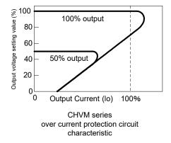
The overcurrent protection circuit shows a drooping characteristic. Ensure that the load to be used is at least with the minimum resistance specified for each series.
