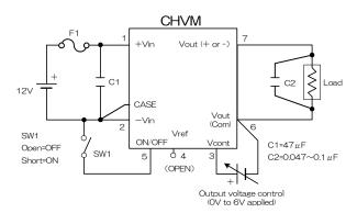
To reduce output noise even further, position C2 near the Load with the shortest input-output wiring while paying attention to creepage and spatial distances.
