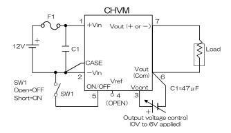
The CHVM series does not basically require additional parts, but add capacitor C1 to the input terminal if input impedance is high due to a long distance between the power supply and converter, an input line is thin, a filter is inserted on the input side, etc. When fitting a capacitor, try to add on the converter terminal side so as to reduce lead inductance.
