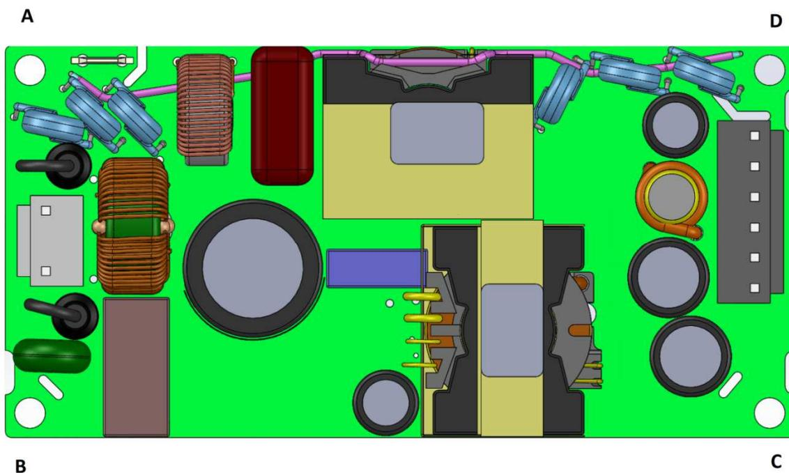
All four mounting points (A, B, C, D) should be used to support the unit.
