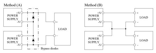
Note: Never use in condition that one of the units is not operated. It will cause power supply to damage. When power supplies are connected as method (A), the bypass diode is required. The bypass diode must be selected with maximum forward current rating and maximum reverse voltage rating of more than output current and output voltage.
