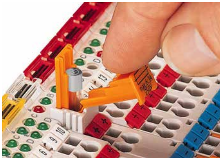
Figure 10: Opening the Fuse Carrier
