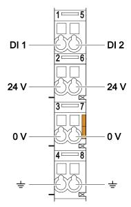
Figure 4: CAGE CLAMP® Connectors
