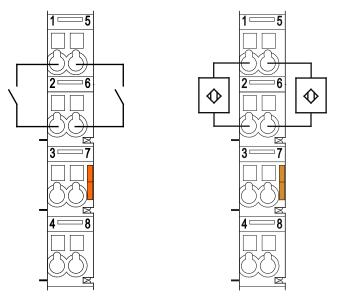
Figure 11: Connecting Diagrams, 2-Conductor Connection
