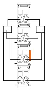
Figure 13: Connecting Diagram, 4-Conductor Connection
