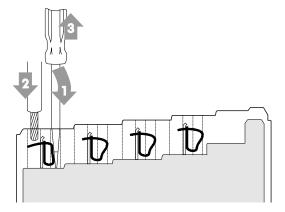
Figure 10: Connecting a Conductor to a CAGE CLAMP®
