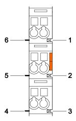
Figure 3: Power Jumper Contacts
