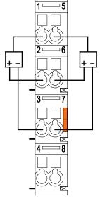
Figure 12: Connecting Diagram, 3-Conductor Connection
