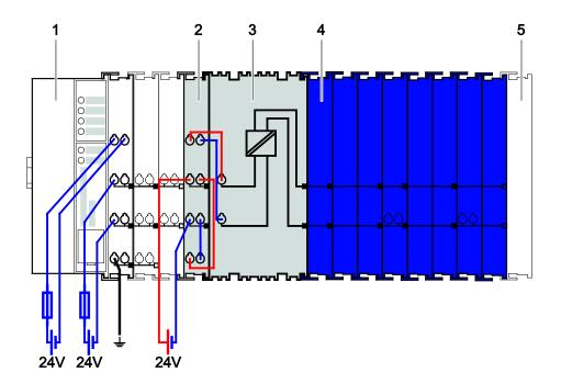
Figure 13: Power Supply Concept, Category EMC1 (Marine Applications)
