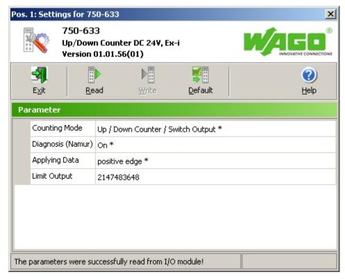
Figure 16: Up/Down Counter Ex i 750-633 (Parameter Dialog Box)
