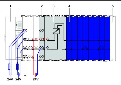
Figure 14: Power Supply Concept, Category EMC2 (Marine Applications)
