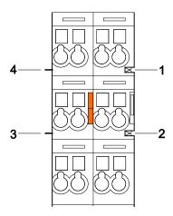
Figure 3: Power Jumper Contacts
