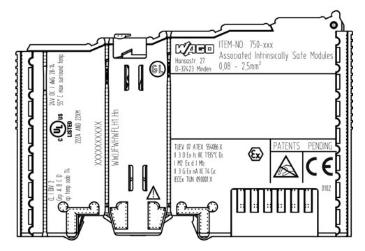
Figure 23: Marking Example According to NEC
