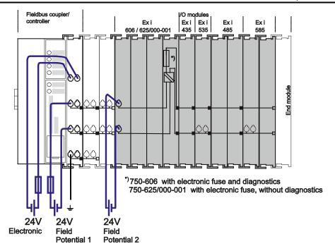
Figure 11: Supply Principle Ex i
