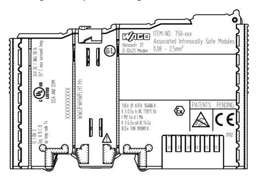
Figure 19: Marking Example According to ATEX and IECEx
