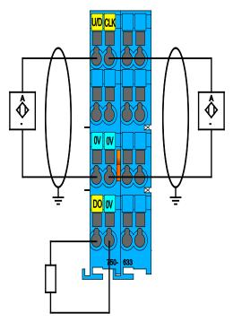
Figure 15: Connection Example for U/D (GATE), CLK and DO
