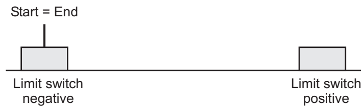
Fig. 2.1.2-31: Referencing to limit switch with start in negative direction from negative limit switch
