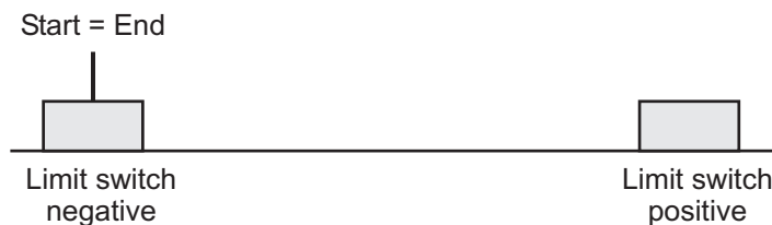
Fig. 2.1.2-32: Referencing to limit switch with start in negative direction from negative limit switch
