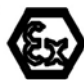
Figure 15: Printing Text detail – Marking example for ATEX and IEC Ex approved I/O modules according to CENELEC and IEC
