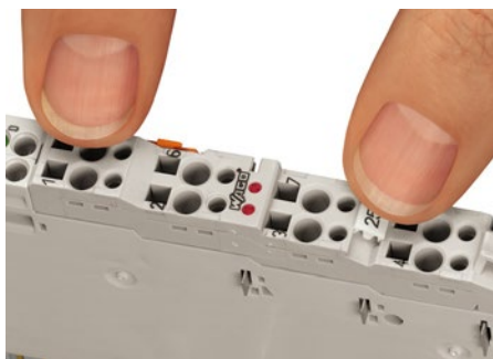
Figure 15: Plugging the Connector into Place
