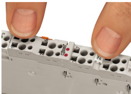
Figure 14: Plugging the Connector into Place
